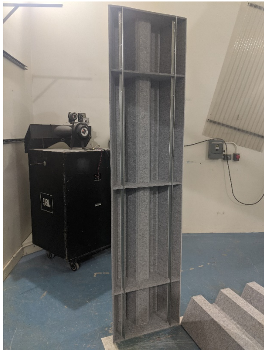
Figure 3 – Underside of individual shell, felt and steel supporting members
