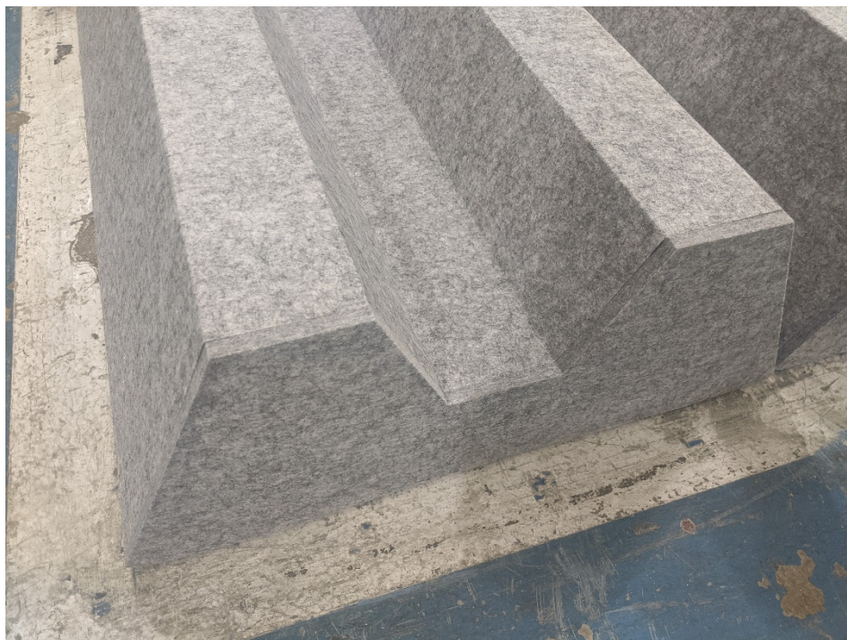
Figure 2 – Detail of specimen material, corrugated profile
